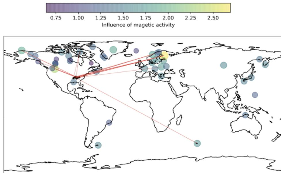
The size and color of the SuperMAG sites indicates the mean influence that each magnetometer has on the TVA sites. The 20 strongest influences are shown as red lines connecting the TVA sites to the SuperMAG sites.
