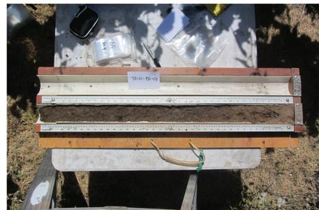
1 meter hand-augered sediment core.
