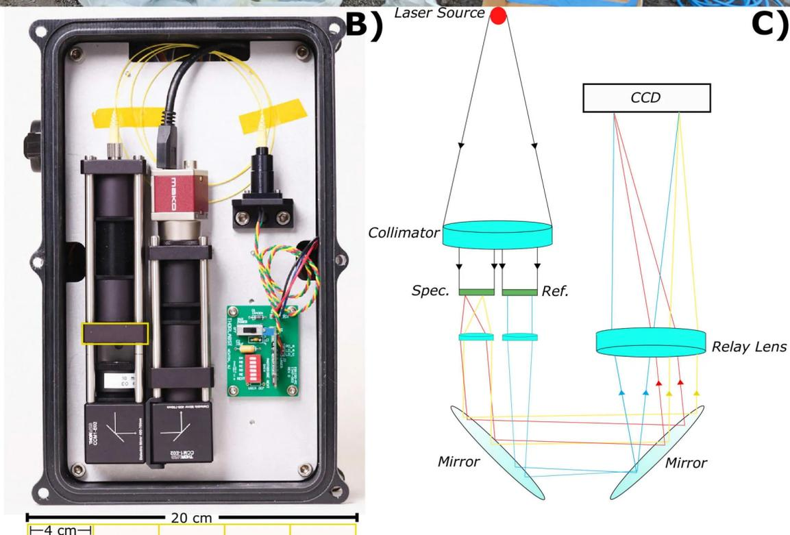
Figure 4. A) A photo of Son of Shamu (SoS) the field deployable DHM being used by Carl Snyder just below the Mount Saint Helens crater. B) Is a photo of a partially assembled DHM allowing use to see the optical train. C) A diagram of the optical components of SoS.
