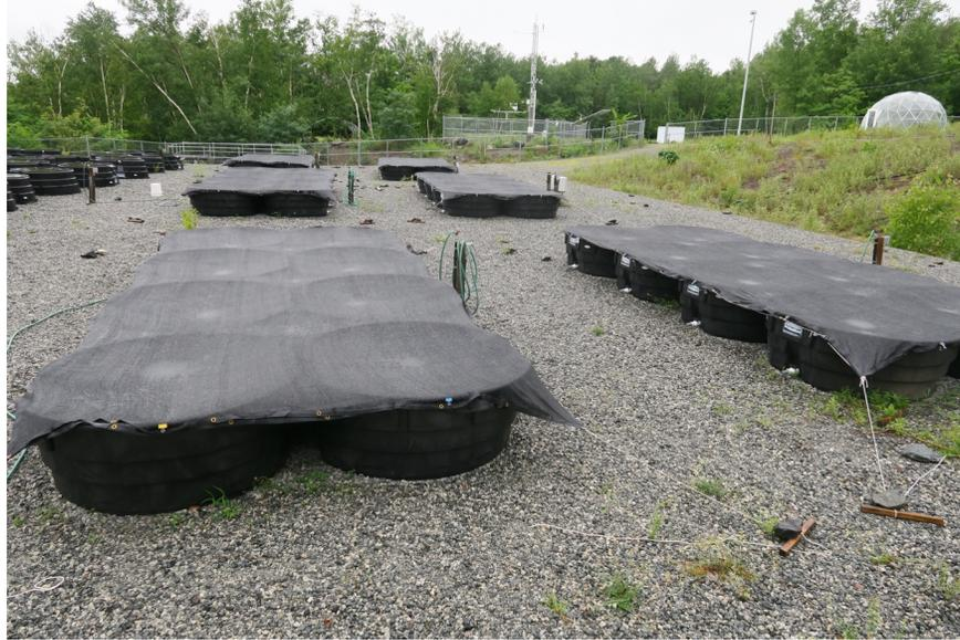
Fig. 1. The experimental setup. 48 mesocosms arranged in six blocks of eight on the LEAP platform at McGill's Gault Nature Reserve. Each block is covered with shade cloth which serves to mimic canopy cover and minimize the input of debris by wind.
