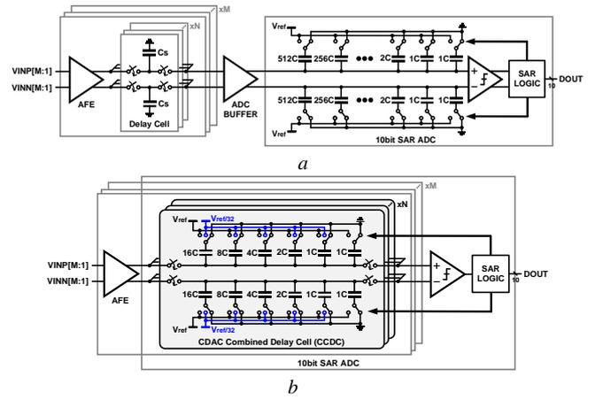
**Fig. 1** Sub-array beamforming RX architecture
