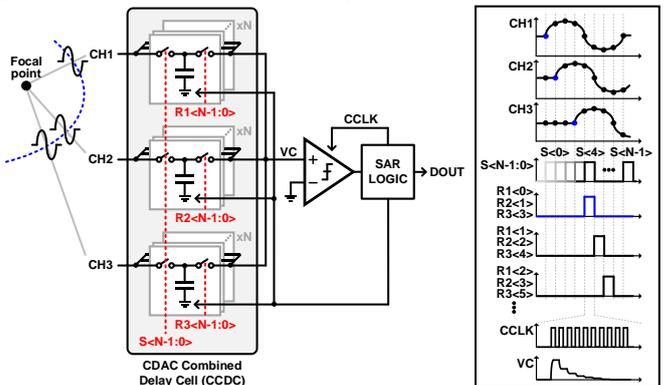
**Fig. 2** Sub-array beamforming SAR ADC with its timing diagram
