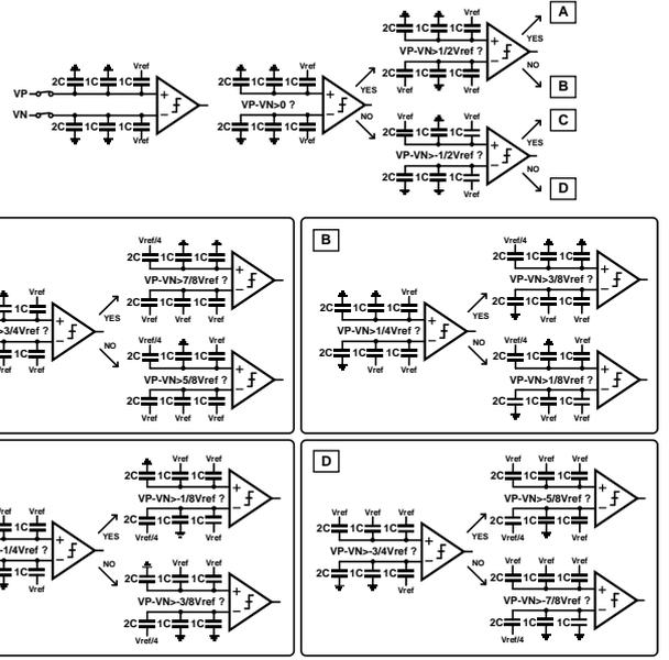
**Fig. 5** Proposed 4-bit switching procedure
