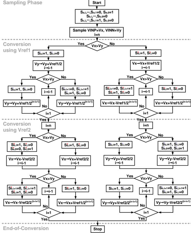
**Fig. 4** Switching flow diagram of CDAC using dual reference voltages
