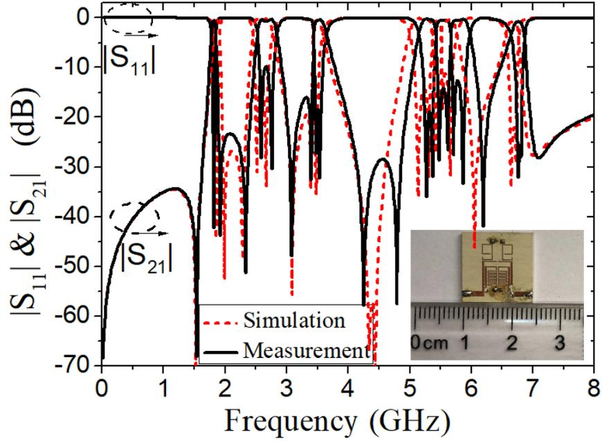
**Fig. 6** Simulated and measured results of sext-band BPF
