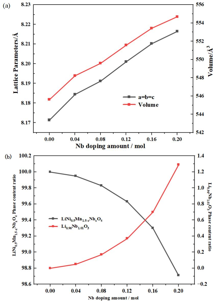
Fig.3. (a) Cell parameters and volume variation curves for different Nb doping amounts; (b) Variation curves of phase content of  $\text{LiNi}_{0.5}\text{Mn}_{1.5-x}\text{Nb}_x\text{O}_4$  and  $\text{Li}_{0.96}\text{Nb}_{1.01}\text{O}_3$  with different Nb doping amounts
