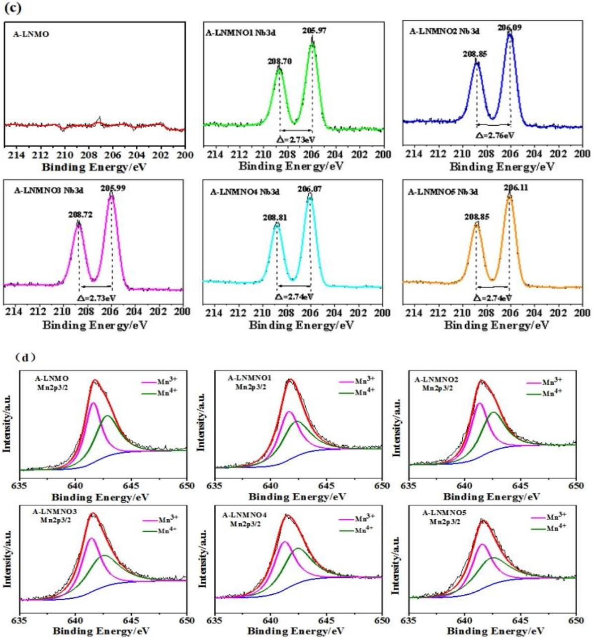
Fig. 6. XPS images of  $\text{LiNi}_{0.5}\text{Mn}_{1.5}\text{O}_4$  and  $\text{LiNi}_{0.5}\text{Mn}_{1.5-x}\text{Nb}_x\text{O}_4$ : (a) Ni2p; (b) Mn2p; (c) Nb3d; (d) Mn2p<sub>3/2</sub> fitting figure
