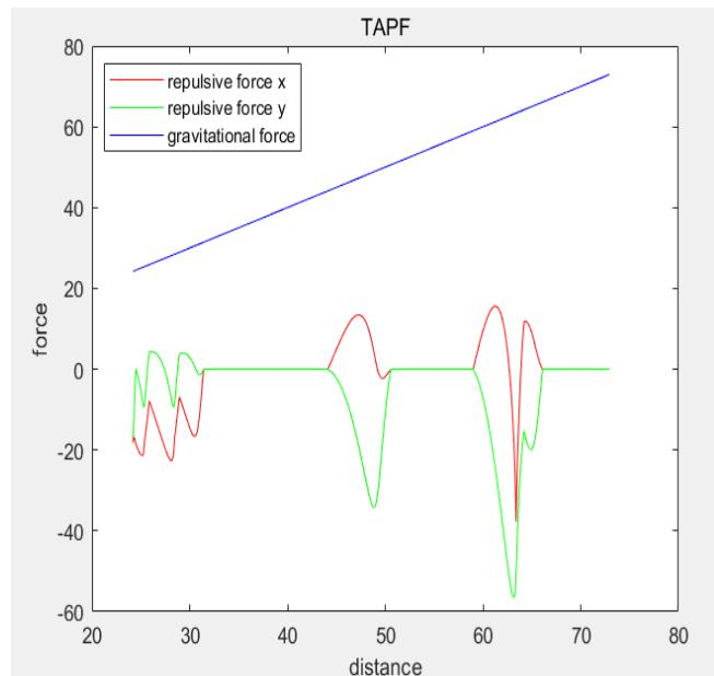
**Fig. 15** TAPF Gravitational and repulsive force changes
