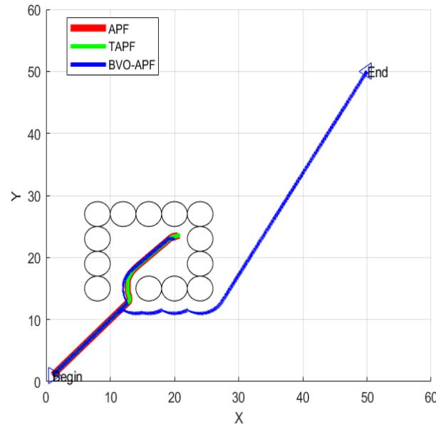
**Fig. 12** Path comparison of three algorithms in U-shaped obstacles
