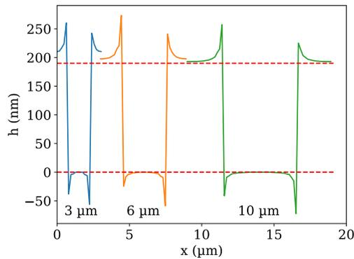
**FIGURE 6** Simulated rectangular profiles of period lengths ( $3\ \mu\text{m}$ ,  $6\ \mu\text{m}$  and  $10\ \mu\text{m}$ ) obtained by use of the Gaussian fit (GF) algorithm. The red dashed lines represent the upper and lower levels corresponding to the nominal height of 190 nm.
