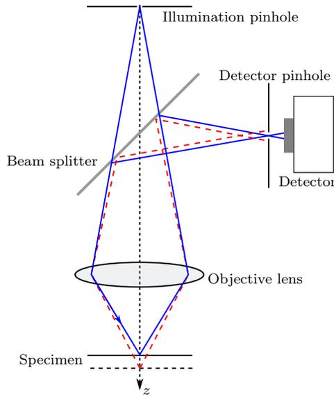
**FIGURE 1** Schematic illustration of a confocal microscope. The blue line illustrates the imaging beam path, if the specimen is in focus of the microscope objective. An out of focus beam path is exemplarily represented by the red dashed line.
