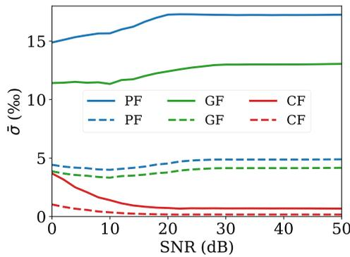
**FIGURE 11** Averaged standard deviations of the fitted curves obtained by the different signal processing algorithms with respect to the simulated intensity signal. The solid lines represent  $\bar{\sigma}$  obtained for a threshold of 0.6 and 0.8 in case of the dashed lines.
