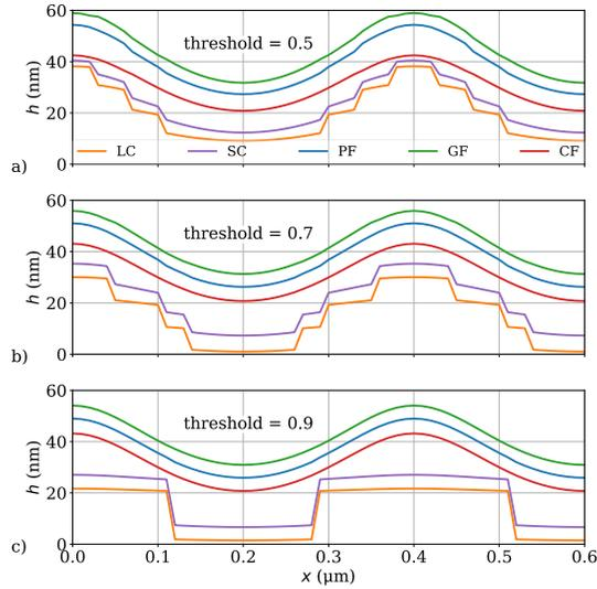
**FIGURE 7** Simulated profiles of a rectangular grating with a period length of 400 nm and a step height of 140 nm. The confocal depth response signals are simulated and evaluated using linear centroid (LC), square centroid (SC), parabolic fitting (PF), Gaussian fitting (GF) and cubic fitting (CF).
