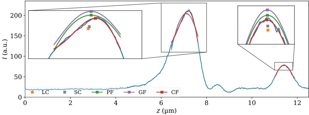
**FIGURE 12** Response signals (blue) obtained experimentally from a layer thickness standard, including the fits of the different fitting algorithms as well as crosses to mark the position determined by centroid approaches. Note that the curves shown in the magnified sections, which are determined by PF and GF as well as the crosses representing the LC and SC approaches, are shifted vertically by a certain offset to improve visibility.
