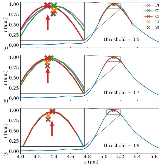
**FIGURE 4** Normalized response signals (blue) obtained from the rectangular structure shown in Fig. 3 at the lateral position  $x = 1.5 \mu\text{m}$ . The axial positions of the correct maximum (see arrow) and the maximum determined by several signal processing algorithms are marked by different colors.
