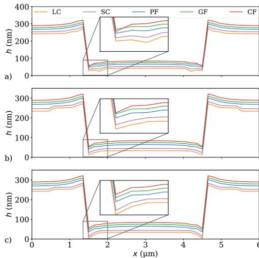
**FIGURE 3** Simulated results from a rectangular surface structure with a period length of  $6\ \mu\text{m}$  and a nominal step height of  $190\ \text{nm}$ . The height values are obtained using linear centroid (LC), square centroid (SC), parabolic fitting (PF), Gaussian fitting (GF) and cubic fitting (CF) for the threshold factors: a) 0.5, b) 0.7 and c) 0.9.
