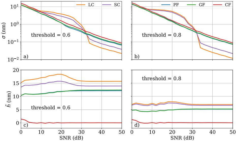
**FIGURE 10** Standard deviation  $\sigma$  of 1000 repeated height values obtained by different signal processing algorithms depending on the SNR of the simulated asymmetric response signals for threshold values of 0.6 (a) and 0.8 (b) as well as corresponding averaged height values  $\bar{h}$  in (c) and (d). Note that all averaged height values are related to  $\bar{h}$  determined by the CF approach for a threshold of 0.6.
