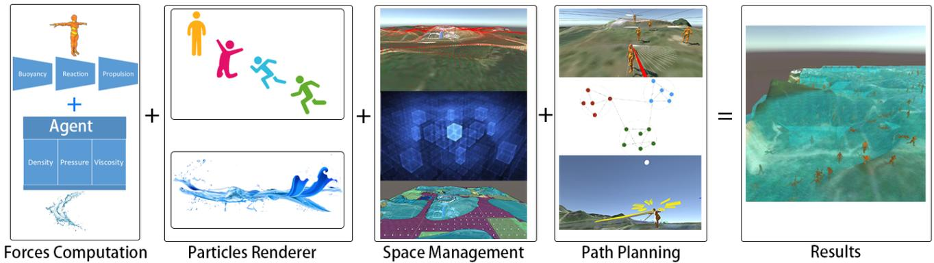
**Figure 1** The overview of our model. Our model treats both the crowd and the water as fluid particles, which allows us to incorporate various forces such as pressure, shear, buoyancy, and active forces to drive the agents. The renderer deals different kinds of particle with different ways. A plane partition method is used to divide the 3D scene into a number of zones. The minimal-rotation path finding algorithm ensure the agent moves toward the destination with the total minimal rotation.
