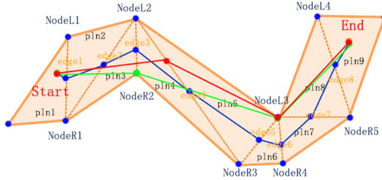
**Figure 2** Comparison of three path planning methods: the midpoint method (blue line), the inflection point method<sup>24</sup> (green line), and our minimal-rotation path planning method (red line).
