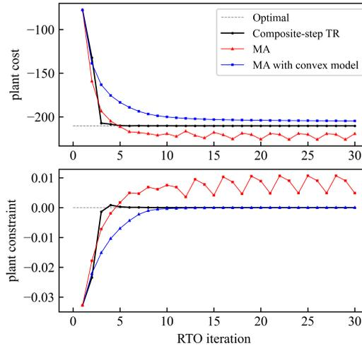
**FIGURE 6** Iteration profile of the William-Otto reactor example
