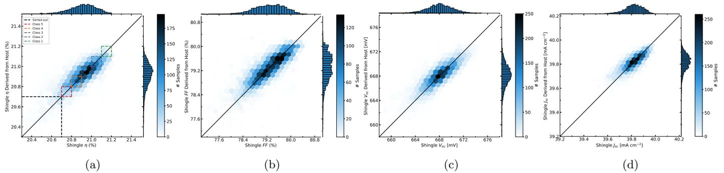
Figure 2: Comparison of the predicted (y-axis) and measured (x-axis)  $IV$  parameters of the shingle cells. In (a) the results are shown with respect to  $\eta$ , in (b) with respect to fill factor  $FF$ , in (c) with respect to open-circuit voltage  $V_{oc}$ , and in (d) with respect to short-circuit current density  $J_{sc}$ .
