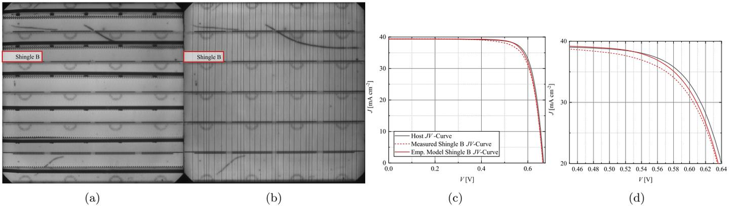
Figure 6: Visualization of the  $JV$  curve calculation of a second example cell. In (a) and (b) EL images of the same host cell are shown, measured with a bar contact unit and the wire-based GridTouch contact unit, respectively. The investigated shingle cell B is highlighted in red. The predicted (red, continuous) and measured (red, dashed) shingle  $JV$  curves and the host  $JV$  curves are displayed in (c) and (d).
