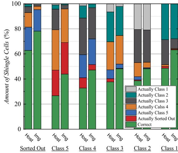
Figure 3: Binning accuracy with respect to the sorting classes using the reference method based on only  $IV$  data of the host cells (left bars) and the our model based on  $IV$  and  $EL$  and  $PL$  image data of the host cells (right bars).
