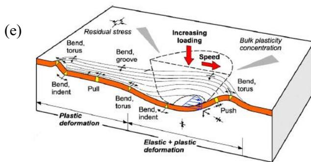
**Fig 2:** Wear track from sliding indentation on CNx coatings on Si (100) substrates and linear profiles of the different failure features (e) the stress field in the coated surface resulting from four loading effects: friction force, geometrical deformations, bulk plasticity concentration, and residual stresses (**reproduced with permission** <sup>10</sup>)
