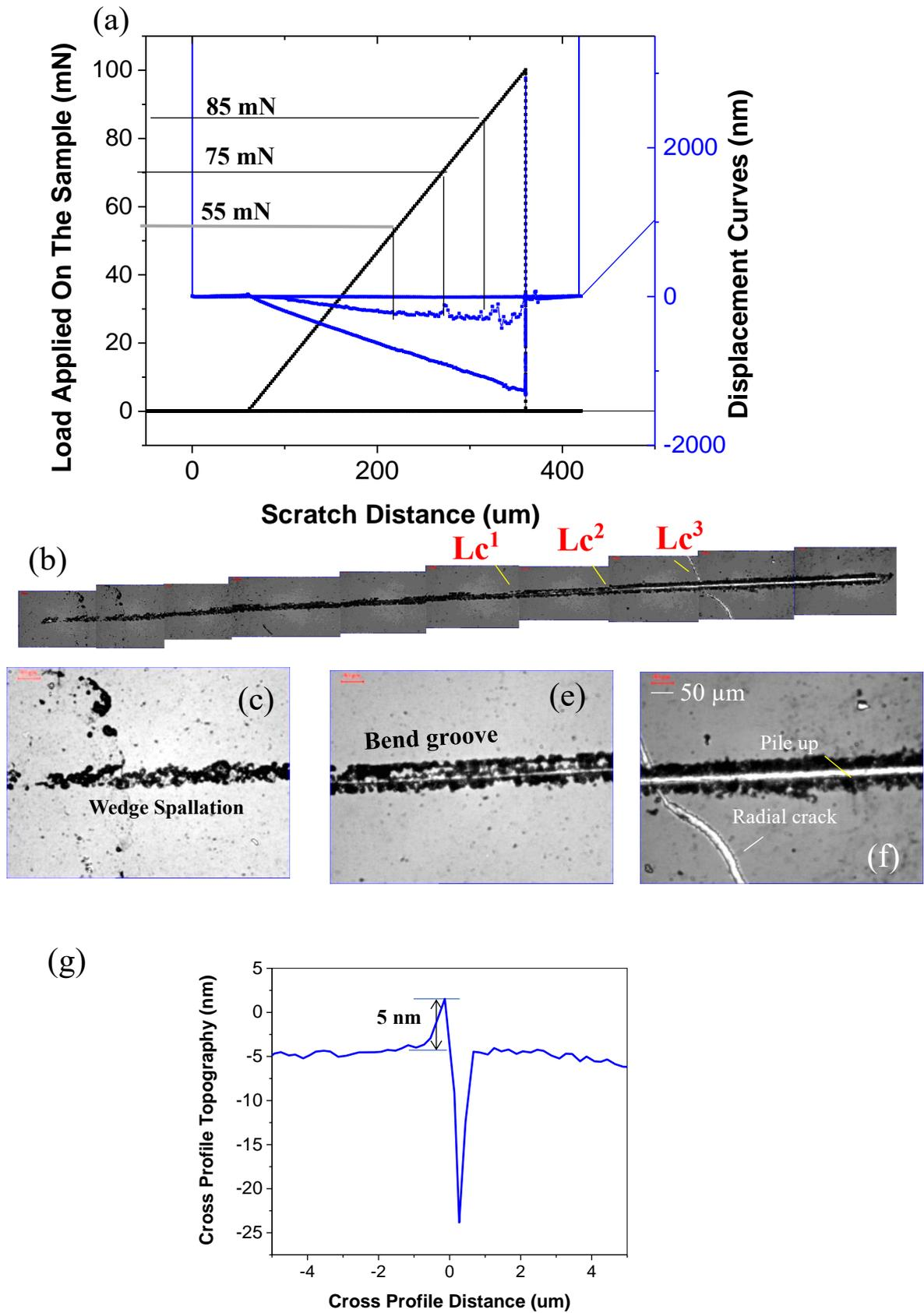
**Fig 2:** Nano scratch test performed on CNx coatings deposited on Si substrates with (a) the 3-stage profiles (b) optical image of the scratch track with (c, d, e) selected magnified area and cross-sectional profile.
