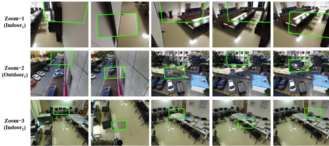
FIGURE 12 The results of our system. The green box indicates the projection of real-time PTZ images in panoramic models. Regions outside green boxes are panoramic models.
